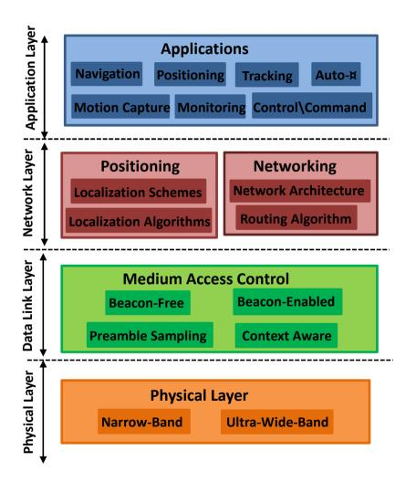
A Wireless sensor networks consists in multiple tiny, low-power and hardware-constrained wireless sensor devices deployed, randomly or manually, over an area of interest to provide a wide range of applications, including weather/environment monitoring, intrusion detection, target tracking, surveillance, etc.
